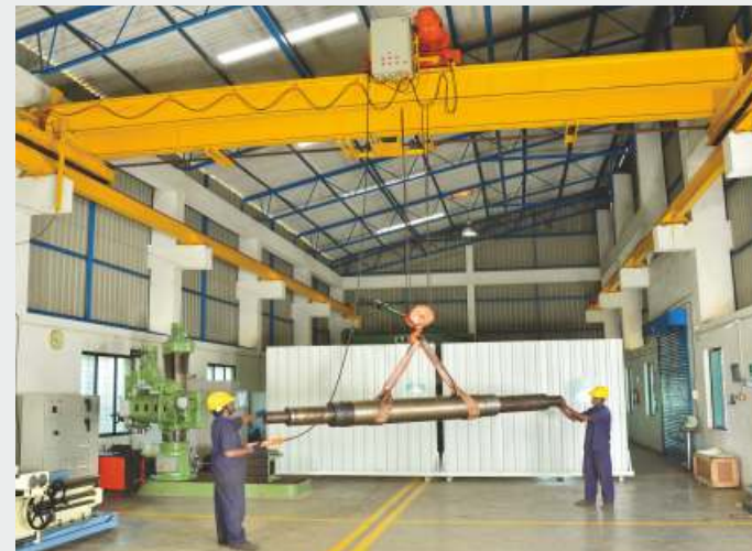
OVERHEAD TRAVELLING CRANE Control: Electrical/Mechanical, Capacity: 10 ton + 5 ton = 15 ton
